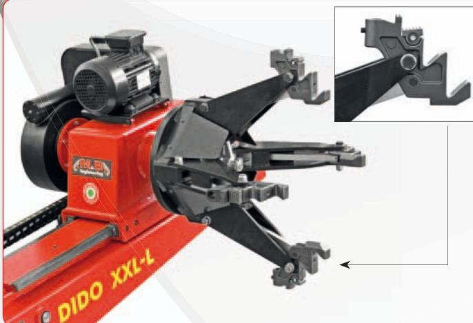
■ Universal hydraulic 4-jaws chuck developed to clamp all types of rims with direct clamp from 14" to 42" (up to 60" using extensions - optional). The new jaw has been designed with 5 clamping points and one of them is adjustable, so that it can be adapted to any type of rim's internal shape. Two speeds for each rotation direction. Central hole minimum diameter clamp: 115 mm.
