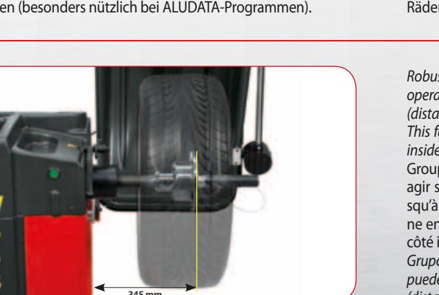
Robust and accurate start up group: typical of a top of the range balancing machine, it can operate on wheels of maximum weight up to 80 kg and with an internal offset up to 345 mm (distance between the wheel mounting surface and chassis) without the use of any spacers. This facilitates inspection of rims/wheels and speeds up the positioning of weights on the inside rim.
