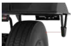
Laser pointer to measure the lateral eccentricity on the tire shoulder.
