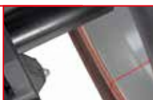
Laser line for the correct application of stick-on weights
